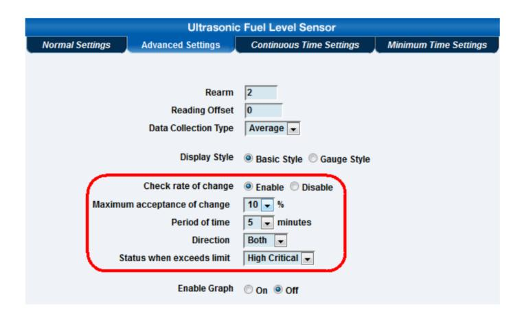
By linking this sensor alert to a notification you can get an SMS, E-Mail, SNMP Alert instantly. This feature is designed for our Ultrasonic Fuel Level Sensor to prevent theft of liquid or be alerted to leaks in storage tanks.
